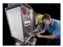
A DEVAP prototype at NREL's HVAC Systems Laboratory
