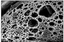
Magnified view of graphene nanocomposite foam
