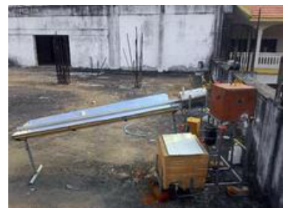
A prototype of a refrigeration system that uses direct sunlight.
