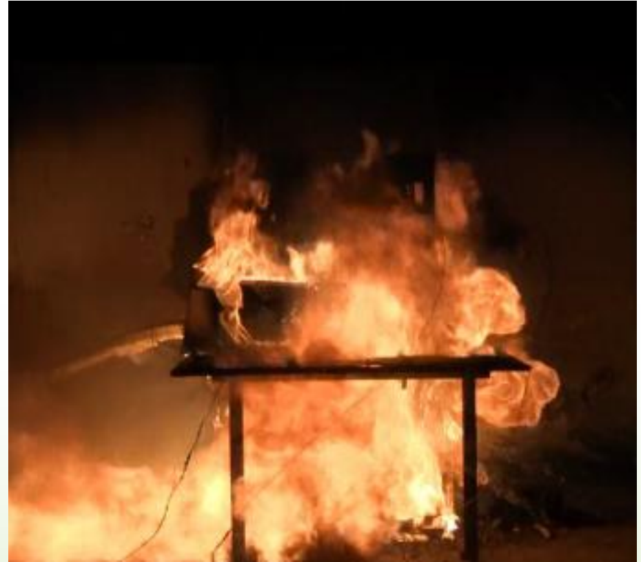
R32 unit combustion experiment
