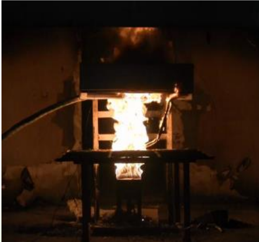
R32 unit combustion experiment
